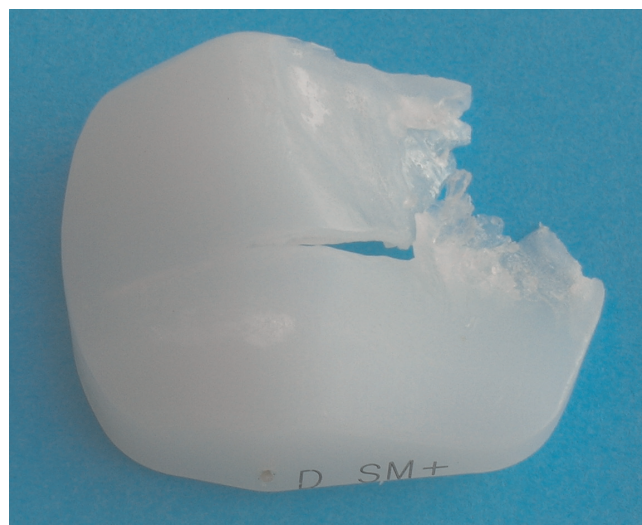
Figure 4. Photograph of the retrieved polyethylene patellar component. The fracture extends radially from the center of the specimen to the markedly thinned superolateral periphery.
