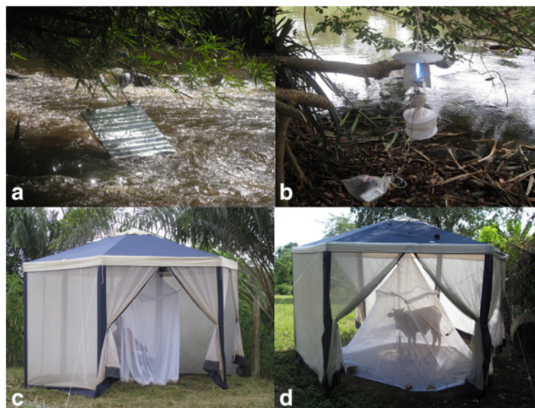
Fig. 2 Methods used to obtain host-independent (a, b) and host-dependent (c, d) adult female blackfly samples. a Bellec (sticky) trap situated above rapids. b Monks Wood (light) trap placed near presumed breeding sites. c Human-baited tent. d Cow-baited tent. a and b illustrate traps to collect ovipositing flies; c and d depict methods to obtain host-seeking flies
