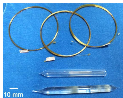
Figure 4. Appearance of PI-coated chromatographic column (CC) samples ( top ) and pristine quartz rods ( bottom ).
