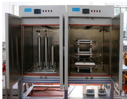
Figure 3. Coreflood setup for evaluating the permeability damage due to different working fluids.
