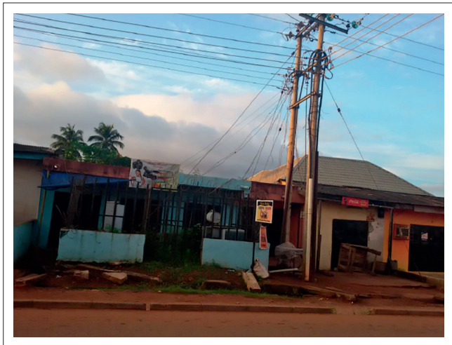
FIGURE 4: A commercial building situated less than two meters behind an 11 000 V transformer.
