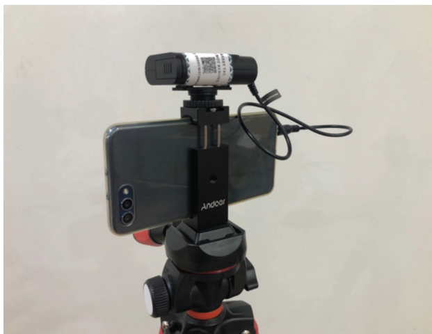
Fig. 1: Android smartphone connected to wireless microphone receiver mounted on a tripod.
