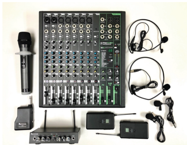
Fig. 2: 12-channel USB Mixer with various wireless microphones and receiver for audio input.
