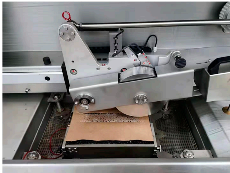
Figure 9. Test facility for the Hamburg wheel-tracking test.
