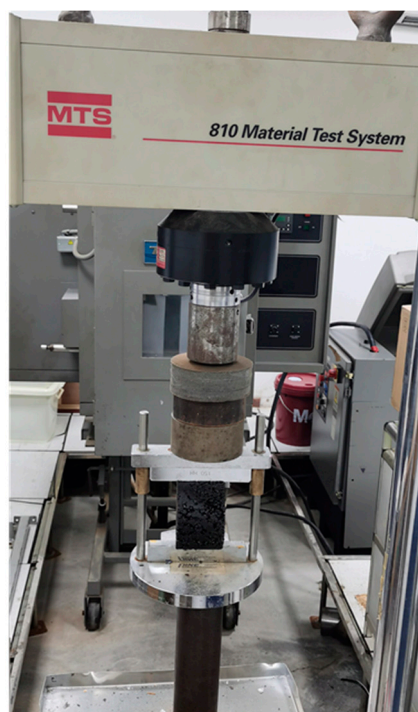
Figure 10. Test facility for resilient modulus test.
