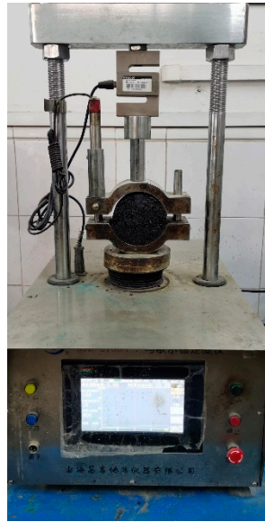
Figure 8. Test facility for freeze–thaw splitting test.
