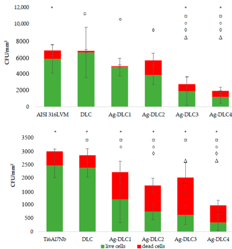
Figure 7. Assessment of microbial colonization of Escherichia coli on Ag-DLC coatings deposited on AISI 316LVM (top) and Ti6Al7Nb (bottom).
