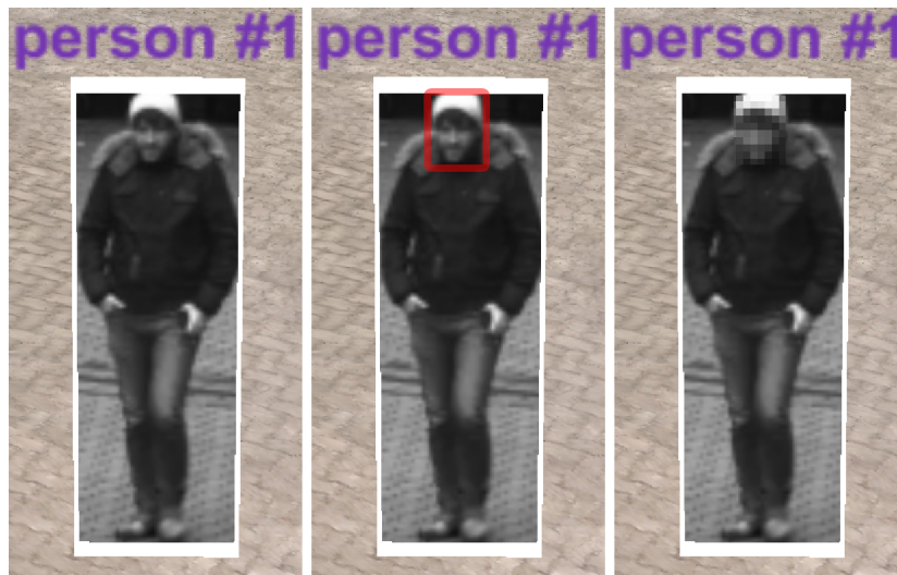
Figure 22. Faces of displayed persons within the 4D reconstruction can be anonymized for privacy reasons. A face detection algorithm detects the bounding boxes of faces ( center ) which are subsequently blurred in the displayed content throughout the visual analysis ( right ).
