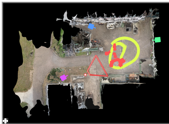
Figure 14. Minimap depicting a top-down view of the reconstructed environment. The locations of the cameras recording the investigated incident are displayed as small camera icons (3 static cameras: blue, green, and magenta; 2 moving cameras: red and yellow). The current location of the user is shown as a small dot, with a red frustum indicating the viewing direction (center) and field of view.
