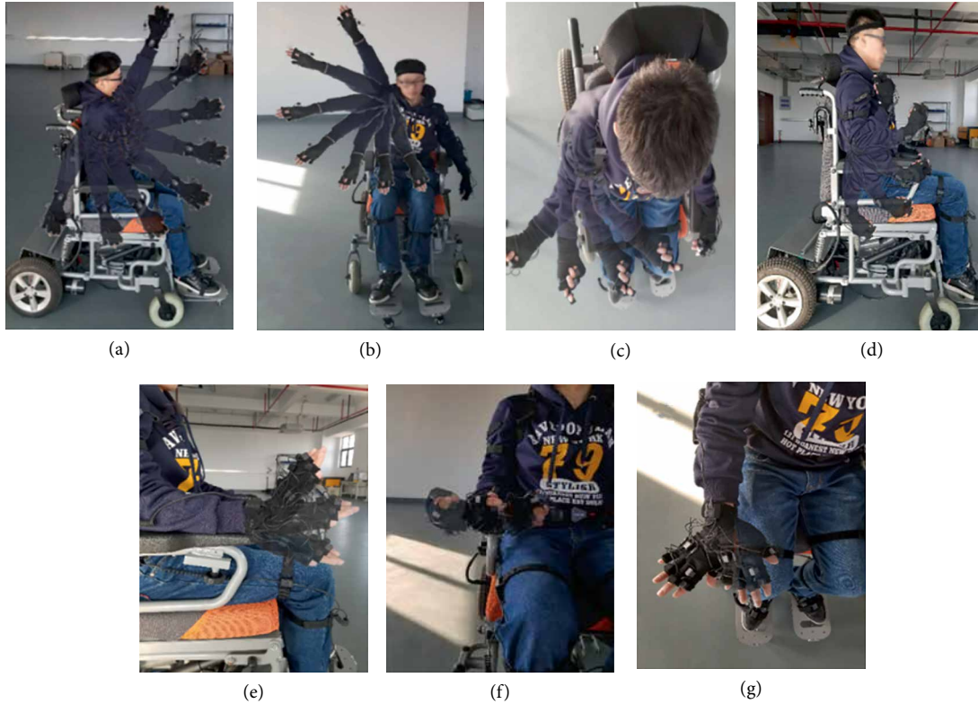
FIGURE 2: The procedure of measuring experiment. (a) Flexion and extension of the shoulder joint. (b) Adduction and abduction of the shoulder joint. (c) Internal rotation and external rotation of the shoulder joint. (d) Flexion and extension of the elbow joint. (e) Supination and pronation of the forearm. (f) Flexion and extension of the wrist joint. (g) Ulnar deviation and radial deviation.
