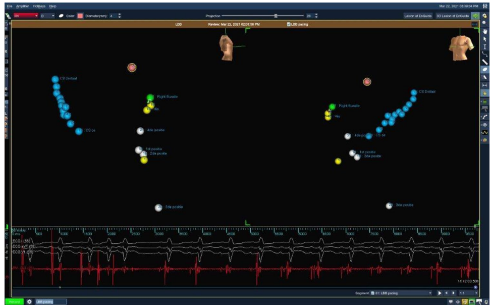
Fig. 1 3-Dimensional electro-anatomical mapping to identify and tag the His-bundle, right bundle region and ostium of coronary sinus. The green dot represents the right bundle branch, the two yellow dots the His bundle and the blue dots the coronary sinus catheter. The divided white dots represent the locations where left bundle branch area pacing was attempted
