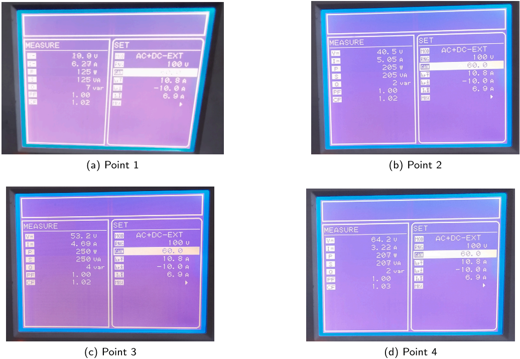
Fig. 18. The output of the power supply on specific points on the I-V curve.
