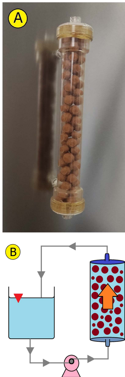
Fig. 1 Nanocomposite ceramics in a fixed-bed column (a) schematic diagram of the adsorption process (b).
