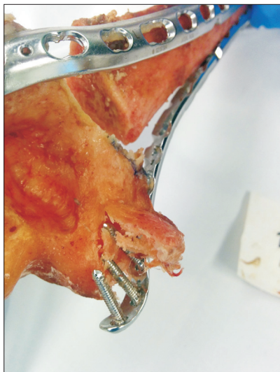
Fig. 5. The locking screws at the distal end of the medial plate broke out of the cortex.
