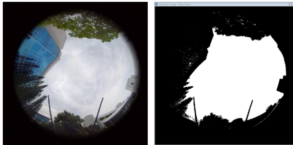
Figure 12. (Left) Photo before Process; (Right) Photo after applying Blue Filter and Threshold Value.
