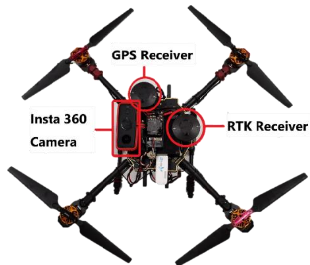
Figure 5. Tarot Ironman 650 with GPS Receiver, RTK Receiver and Insta 360 Camera Facing Upwards.
