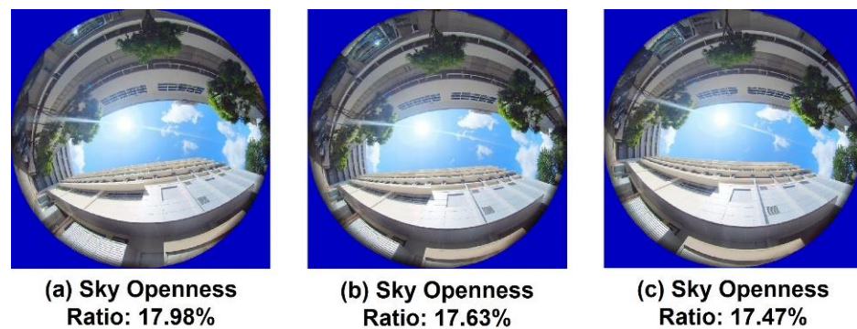
Figure 13. Hemispheric Photo Taken at 1 m Apart near N3.1 to Illustrate the (Lack of) Sensitivity of Sky Openness Ratio to Small Variation in Photo Position Relative to the Designated Photo Points.
