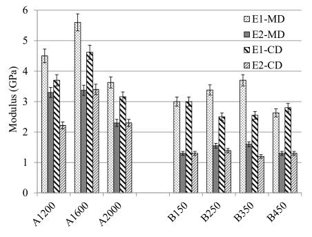
Figure 4. The tensile modulus of A and B nonwoven sets reinforced composites.
