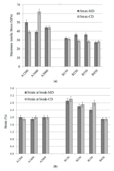
Figure 3. Tensile stress (a) and strain at break (b) for A and B set nonwovens reinforced composites.
