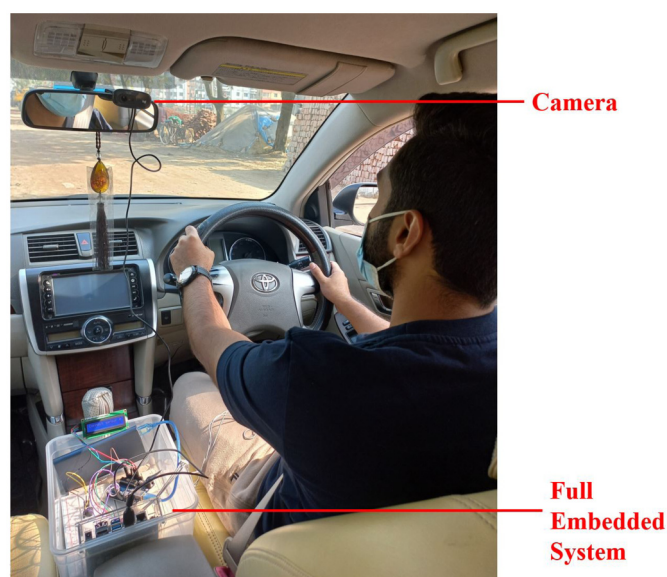
Fig. 39. Illustration of full embedded setup of the proposed driver drowsiness detection system.
