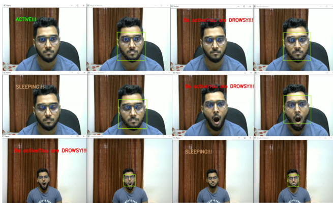
Fig. 30. States classification from varying distances with eyeglasses.
