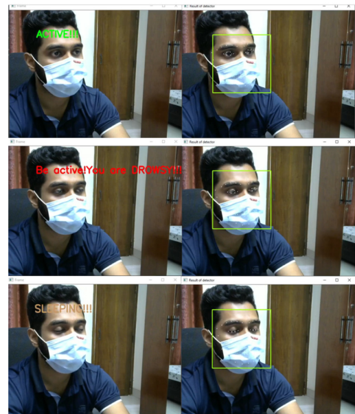
Fig. 32. States classification with the face mask in oblique projection.
