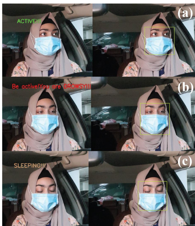
Fig. 37. States classification for real-life experiments with wearing face masks; (a) Active, (b) Drowsy and (c) Sleeping states.
