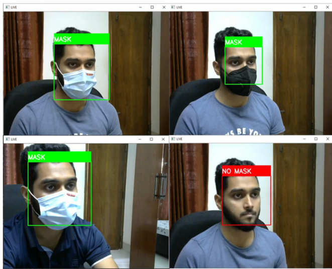
Fig. 24. Successful predictions of face mask detection model in oblique projection.
