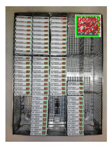
**Figure 5.** The reading process of barcodes directly from the rack containing the blocks during the processing phase after the digital transition. In the upper right inset the code extracted from the 2D barcode directly in the LIS.
