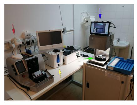
**Figure 7.** An example of a sectioning station. The technician can identify the block through a barcode reader (red arrow), entering the LIS page of the case and printing the related glass slides with a laser printer (yellow arrow). After sectioning, the technician can directly scan the cut surface positioning the block on the dedicated space in the BlocDoc instrument (green arrow), with the possibility to assess the preview of the obtained image (blue arrow).
