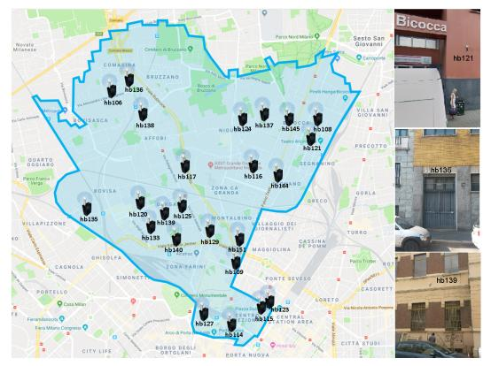
**Figure 3.** Map of the location of the 24-nodes of the WASN deployed within the DYNAMAP's urban pilot area across the District 9 of Milan (**left**), showing the exact installation of three of them in the building facades (**right**) for illustrative purposes.
