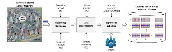
**Figure 1.** Block diagram of the generation process to develop a labelled Wireless Acoustic Sensor Network (WASN)-based acoustic database, where the labels are Anomalous Noise Event (ANE), Road Traffic Noise (RTN) and complex (CMPLX), denoting the latter complex audio passages.
