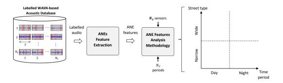
Figure 2. ANE feature analysis methodology from a labelled WASN-based acoustic database.
