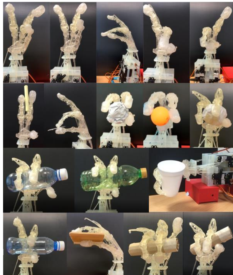
Figure 10. Tasks. Row 1 presents the performance of five Kapandji tests. Rows 2–4 show the robotic hand performing 12 gestures from the grasping taxonomy.
