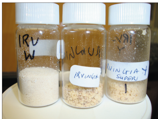
Figure 1: Irvingia fractions (L-R): White lipid fraction (float), aqueous (middle) and yellow lipid (sediment)
