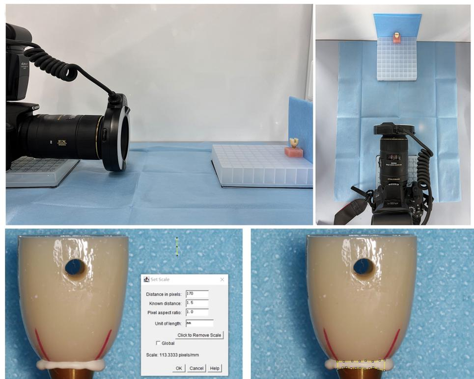
**Fig 3.** (A) Photographing the cemented crowns at a set photo studio and (B) ImageJ evaluation process for the calibration and calculation of the distributed cement extrusion areas.
