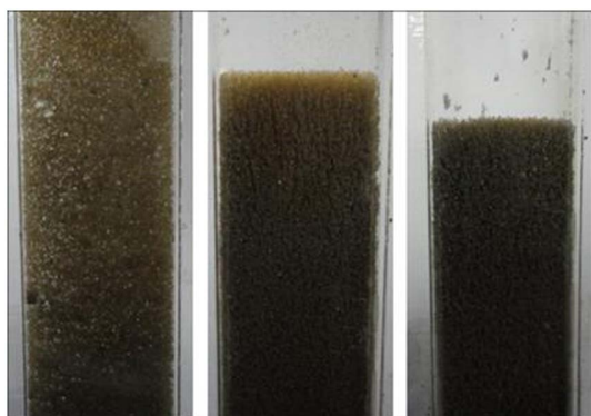
Figure 5 | Photographs for the MS-PSD acid resin catalysts in (a) the scattered particulate state, (b) the chain state, and (c) the magnetic condensation state. The strengths of the applied magnetic field are 0, 30, and 50 \text{kA m}^{-1} for (a), (b), and (c), respectively. To show these operation states, the tube accommodating the catalyst was made of transparent PMMA rather than stainless steel that is used for the reactor, and the fluid was changed to the colorless water rather than the yellowish FCC light gasoline for clarity. The liquid hourly space velocity (LHSV) was 1.0 \text{ h}^{-1} , similar to the typical value for the etherification of FCC light gasoline.
