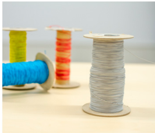
Figure 1. Piezoelectric PLLA braided cord.
