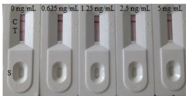
Figure 7. Result of CIP detection via the colloidal gold immunochromatographic strip assay (ng/mL) in spiked milk (n = 6). T, test line. C, control line. S, sample.
