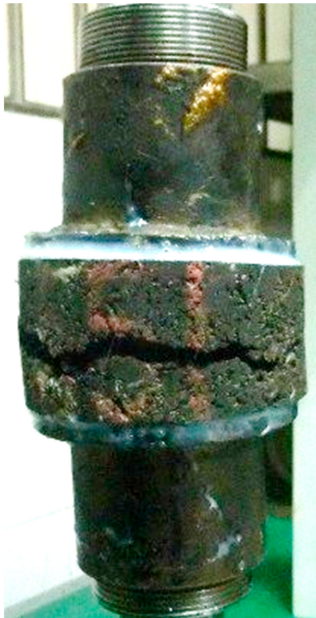
Figure 2. Tensile sample and pulling heads.
