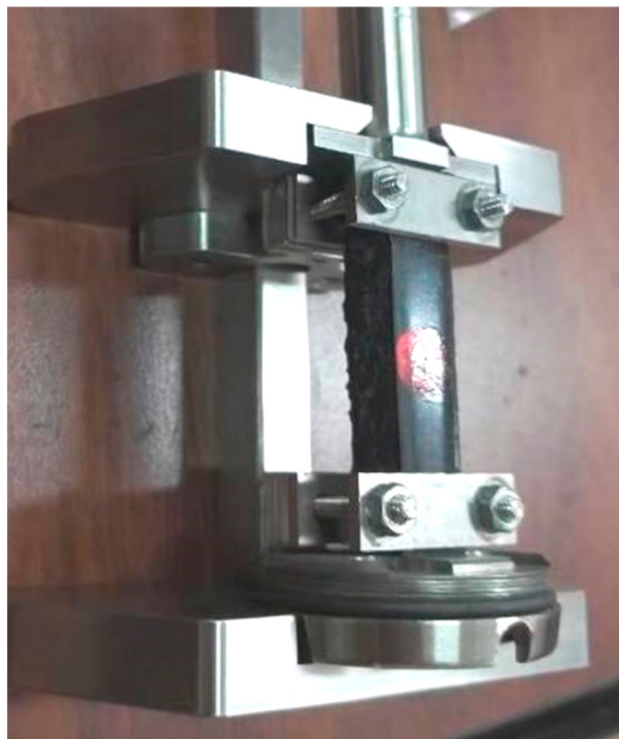
Figure 1. Dynamic shear test sample and fixture.
