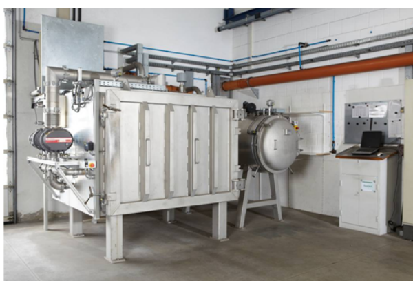
Figure 7. (Oxy-)fluorination chamber used for the treatment of the technical fibers, with permission from Fluor Technik System GmbH.
