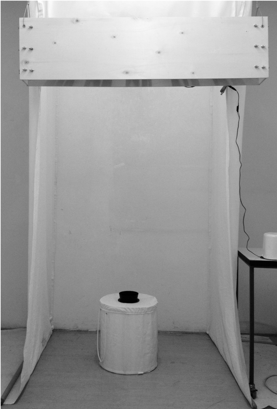
Fig 1. Laboratory test set-up showing the tent structure, BGS trap and FFS (front view).
