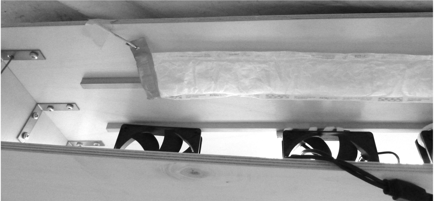
Fig 2. Stericlin repellent sachet attached to the FFS with the permeable side facing the fans.
