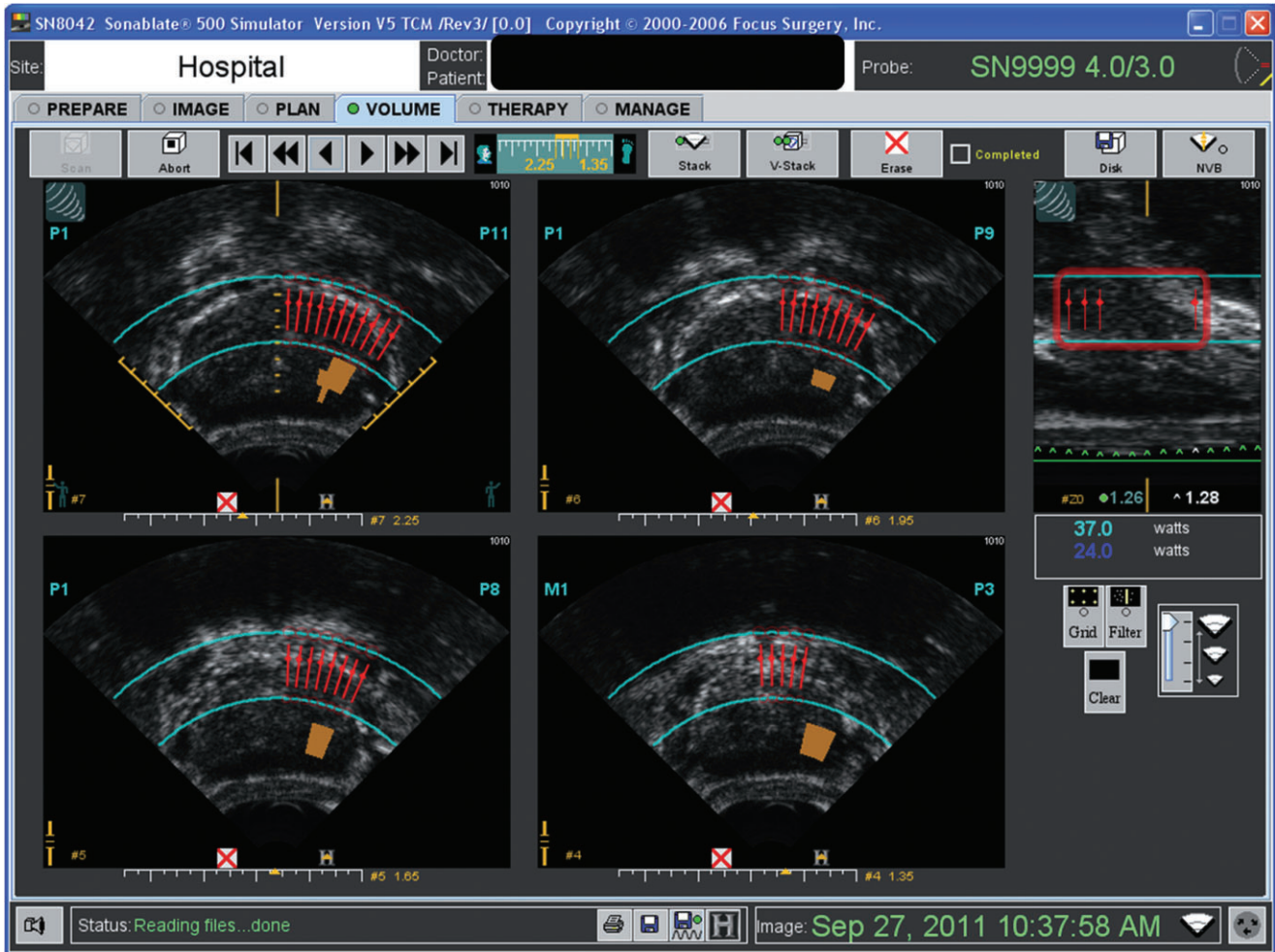
Fig. 4 Screenshot from the HIFU therapy planning software: A visual representation of the target lesion volume is displayed as a coloured (yellow) overlay on the TRUS images on the HIFU workstation. The red lines define the region to be treated.
