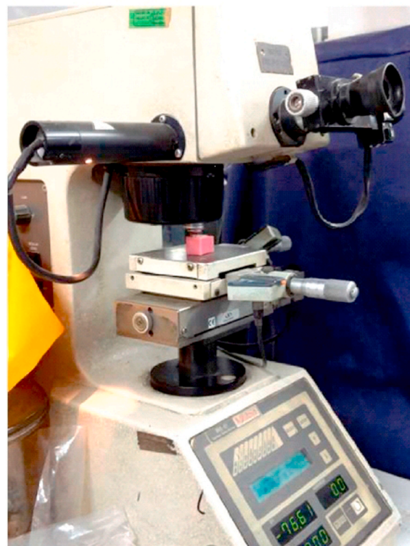
Fig. 7image showing Vickers microhardness tester assessing baseline microhardness.
