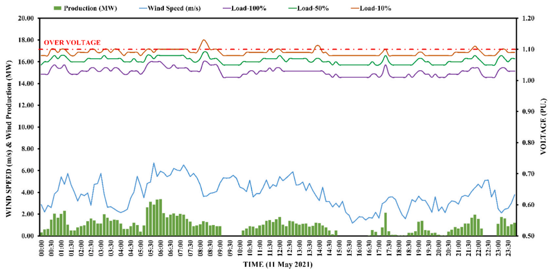
Fig. 17. Selected feeder trip day from May with different load conditions.
