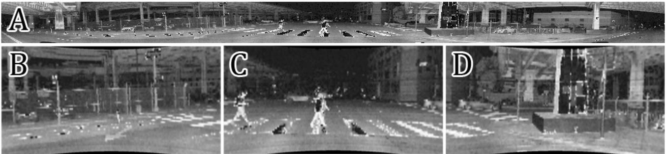
**Figure 2.** Comparison of a directly generated laser intensity image from Ouster OS1-64 (A), and the camera-like images (B–D) for the same scan from one of the publicly available OS1-64 sequences synthesized with our algorithm.
