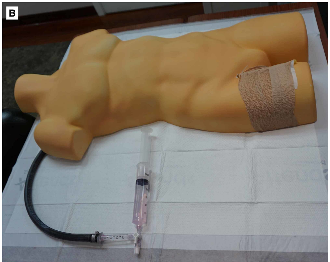
FIGURE 4: Completed REBOA insertion trainer. The rubber tubing (used to simulate the femoral artery) is covered and
