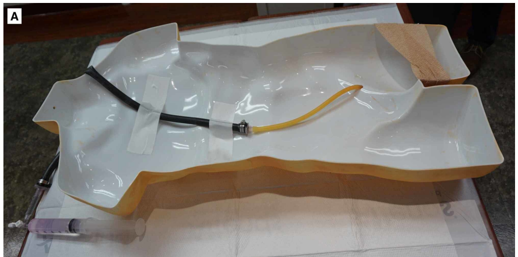
FIGURE 3: Completed REBOA insertion trainer. The REBOA model is attached to the underside of a human torso mold, with the caudad end passing through the torso at the inguinal region.
