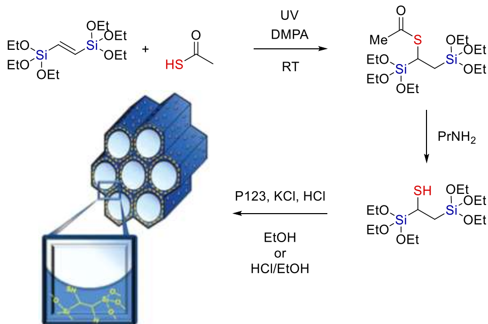
Figure 8. The synthesis of 1-thiol-1,2-bis(triethoxysilyl)ethane (2) and the corresponding thiol-PMO (SH-PMO). Adopted from Ref. [35].
