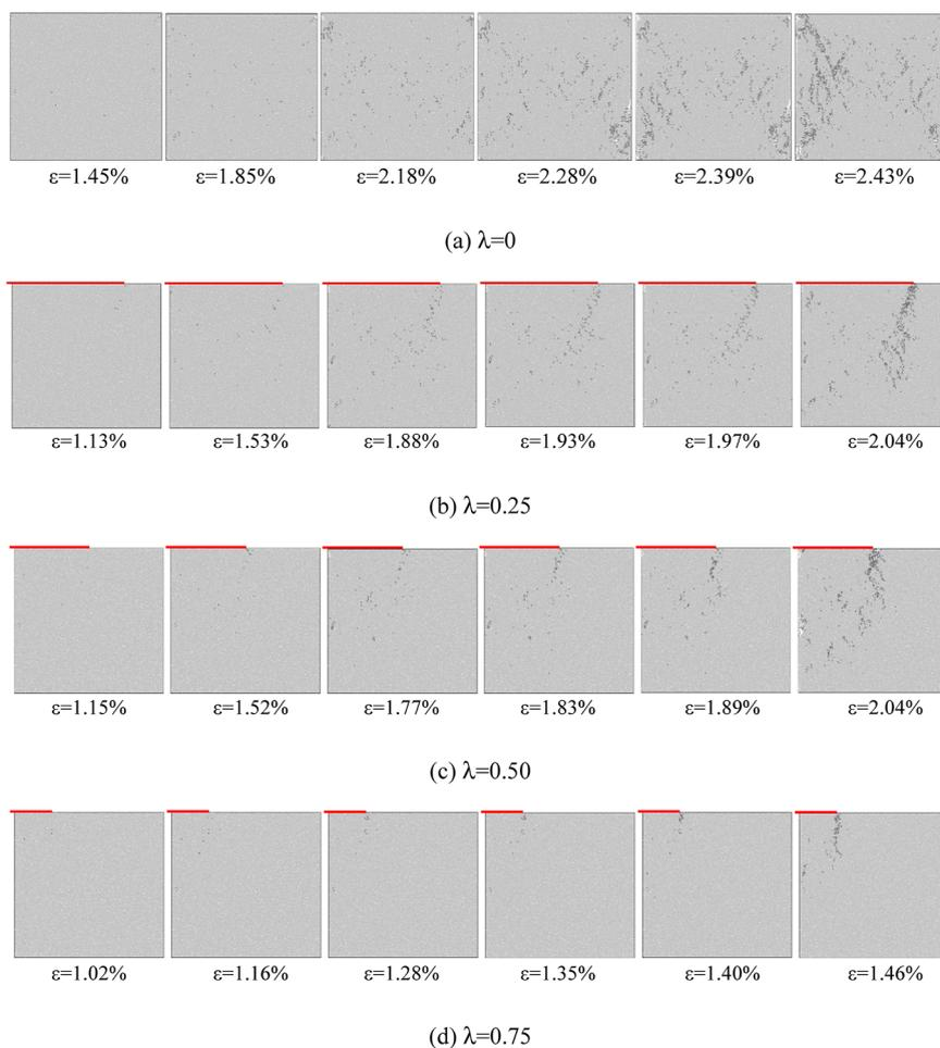
**Figure 9.** Surface crack distribution characteristics of samples at different loading times. (a)  $\lambda = 0$ , (b)  $\lambda = 0.25$ , (c)  $\lambda = 0.5$ , and (d)  $\lambda = 0.75$ .
