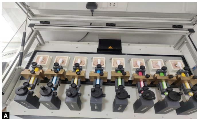
Figs 2A and B: Toothbrush simulator (SD Mechatroix) (A) During brushing simulation; (B) After brushing simulation
