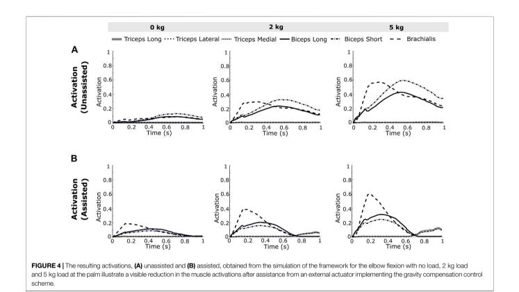
*External load in hand*: An external mass has been attached at a distance of 29 cm from the elbow joint, as shown in **Figure 2**. The mass of this load is varied (0, 2, 5 kg) to observe the rise in muscle activation patterns and subsequently, the reduction in the muscle activity after incorporating actuator assistance.
