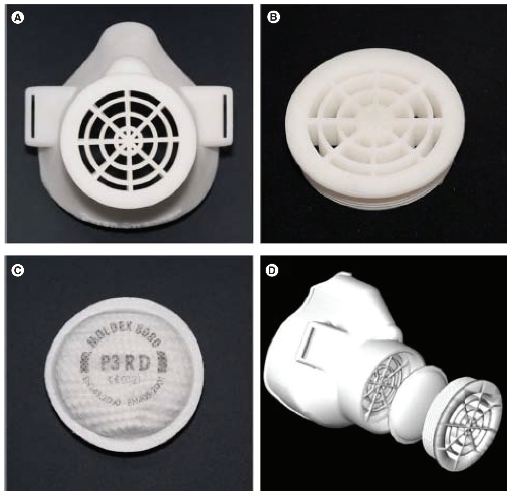
Figure 1. Individualized custom-made 3D-printed protective face mask. Reprinted with permission from [26] © Elsevier (2020).
