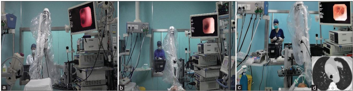
Figure 2. Research of Robotic system of bronchoscope developed for COVID-19 patients. (a) Robotic system in tracheobronchial tree model. (b) Robotic system in animal model. (c) Robotic system in patient. (d) Computed tomography of the patient
