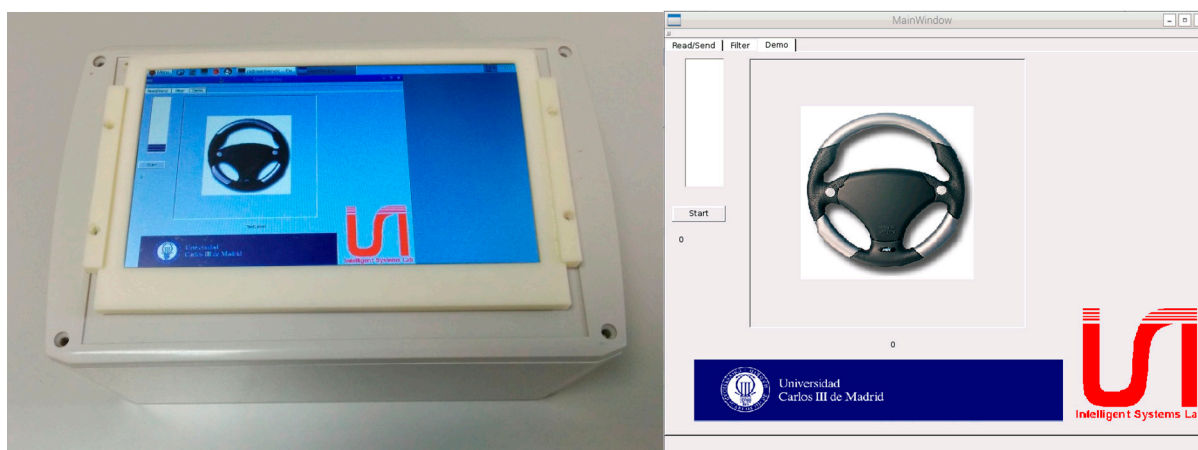
Figure 5. Full driver monitoring system module (a) system with the display mounted; (b) Example of real time steering wheel angle and throttle display.
