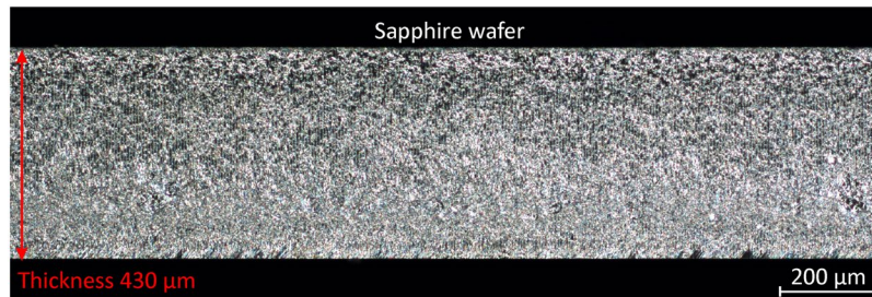
Figure 5. Image of a sapphire sidewall after laser dicing. The dark field optical microscope image of the fracture plane containing subsurface modifications induced by the dual-wavelength double-pulse laser irradiation. Four layers of merged modifications at different focus depths formed a uniform fracture plane. The lateral spacing between the laser-induced modifications was 6\ \mu\text{m} . Processing parameters: HWP orientation angle \varphi = 15 degrees; UV pulse energy E_{p355} = 2.2\ \mu\text{J} ; IR pulse energy E_{p1064} = 51.5\ \mu\text{J} ; scanning speed 600\ \text{mm/s} ; laser pulse repetition rate 100\ \text{kHz} ; pulse duration 10\ \text{ps} ; time delay \Delta t \approx 0.1\ \text{ns} between pulses (UV prior IR); number of scans 4; focal position difference in each of the scan 90\ \mu\text{m} ; total dicing speed 150\ \text{mm/s} .
