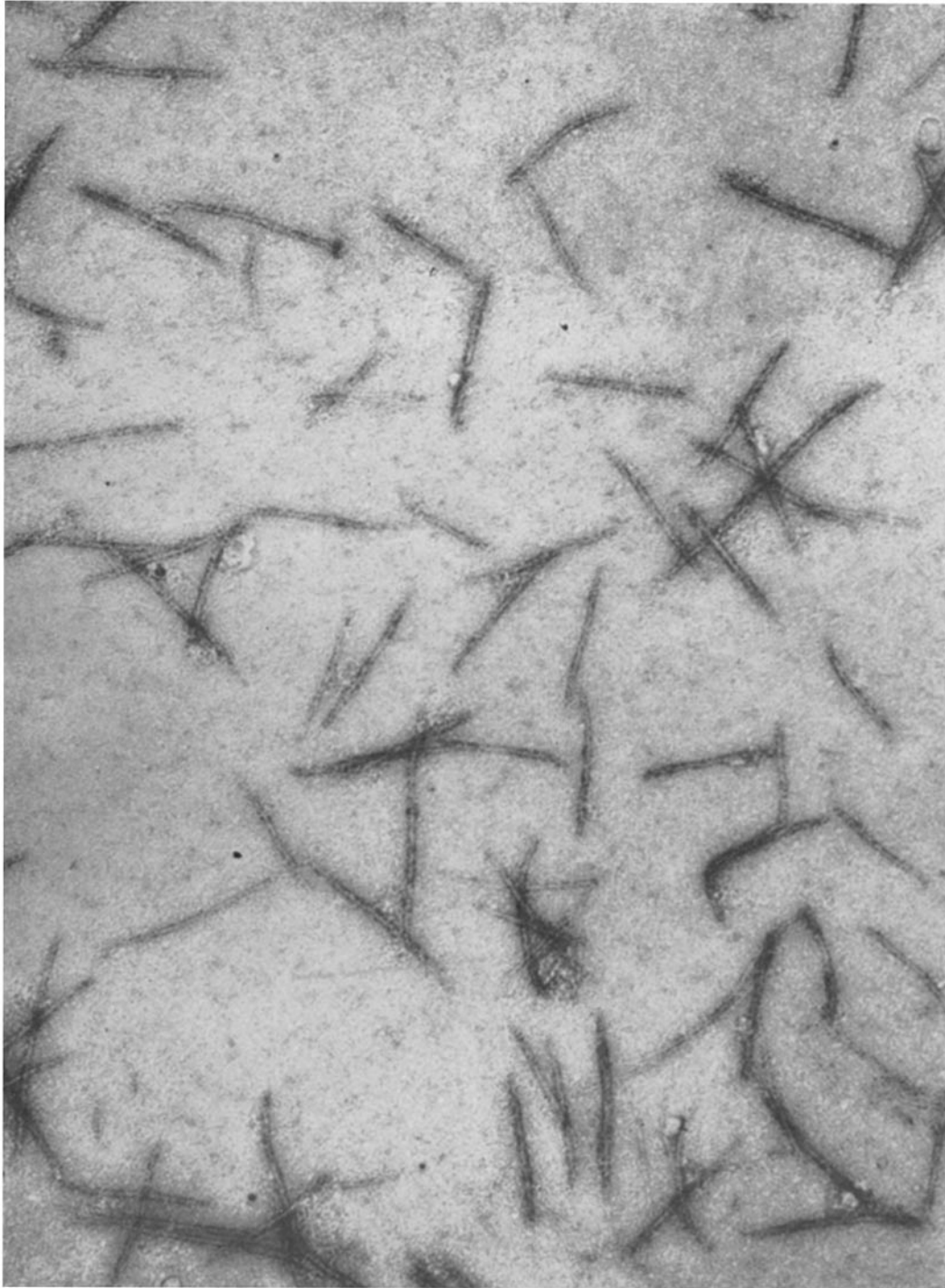
FIGURE 8 Spindle-shaped aggregates, prepared by slow dilution of ultracentrifugally pure canine cardiac myosin in potassium chloride ( \mu = 0.6 ) with standard potassium chloride ( \mu = 0.15 ), negatively stained with 1% uranyl acetate. Aggregates are about 0.5 to 1.0 \mu in length and 50 to 100 \text{\AA} in diameter. \times 32,000 .
