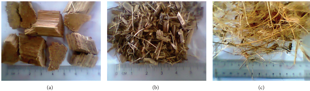
FIGURE 2: OPF feedstock particle sizes resulting from chipping (a) blocks 20 mm × 20 mm × 20 mm, (b) small particles of size less than 10 mm, (c) fine fibres.
