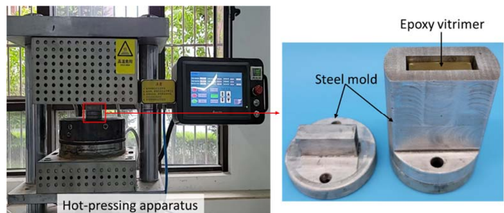
Figure 3. Experimental setup for welding.
