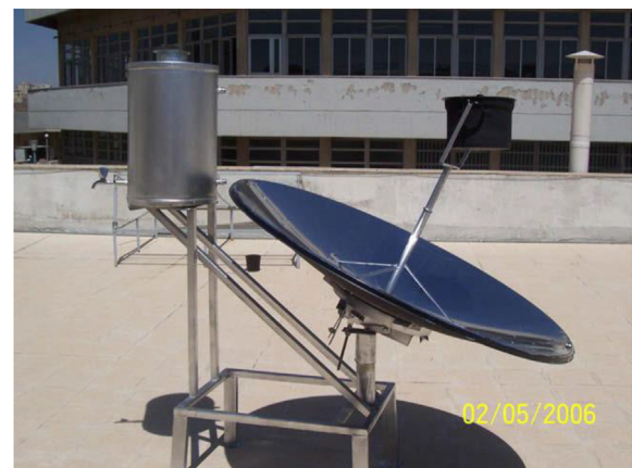
Figure 5. A photograph of the experimental setup of a portable solar cooker and water heater. The figure was reproduced from Ref. [73], with the permission of Elsevier Publishing.
