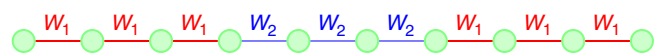
Fig. 1 Illustration of an alternating sector chain (ASC). This example has sector size n = 3 , length N = 10 , and number of sectors 2b + 1 = 3 . Red lines denote the heavy sector with coupling W_1 , blue lines denote the light sector with coupling W_2 < W_1
