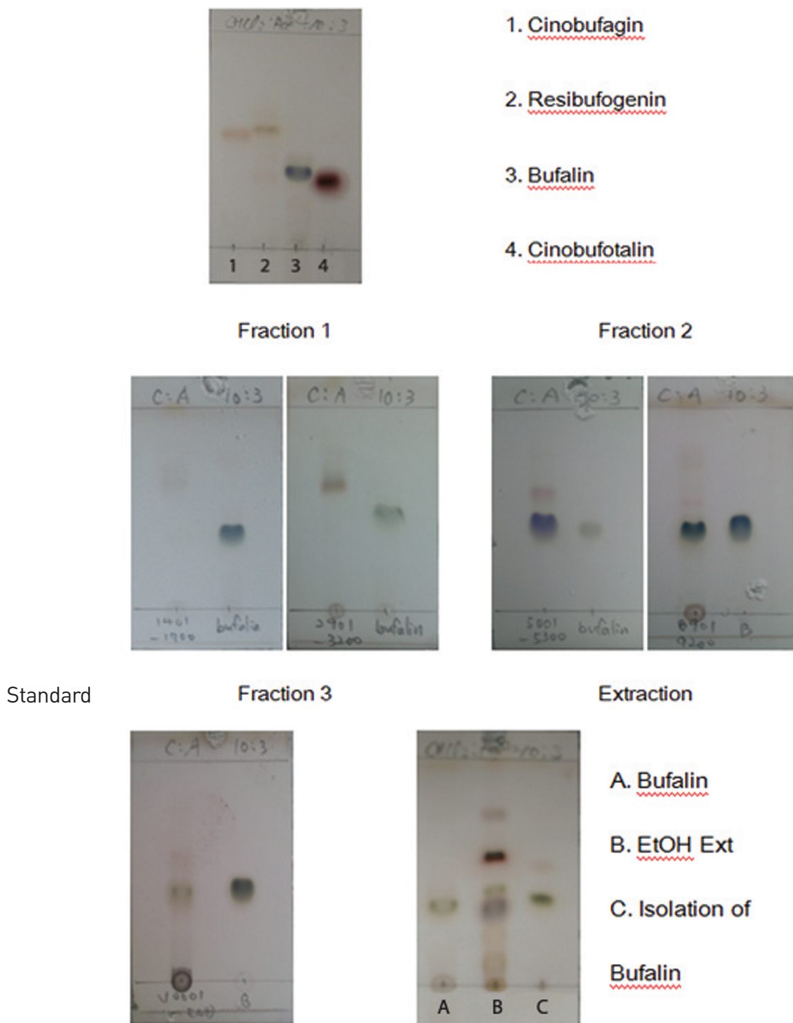
Figure 5 Comparative TLC chromatography results for Venenum Bufonis(plate: TLC silica gel 60 F 254 , developing solvent: CHCl 3 : acetone = 10 : 3, and detection: 10% H 2 SO 4 : 10%).
