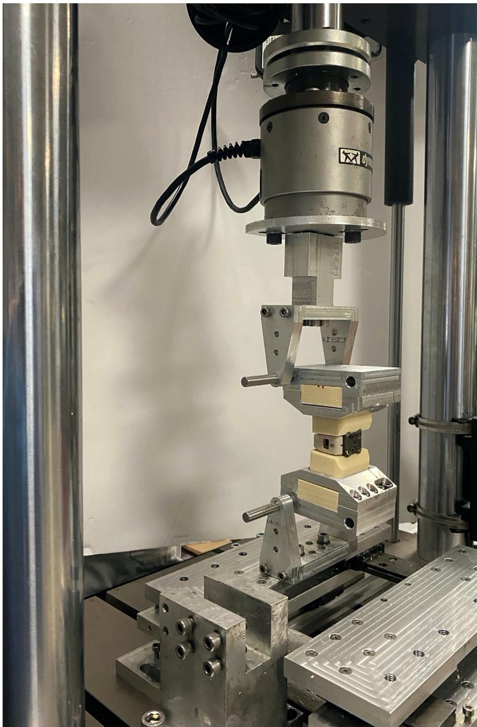
**Fig. 1.** Experimental setup used to load the bone surrogates in a simulated spine extension.
