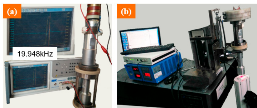
Figure 2. Performance test of the stepped horn: (a) actual resonance frequency; (b) actual vibration amplitude detection.
