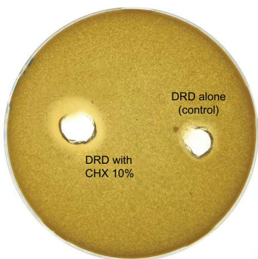
Figure 4 Zone of inhibition of Candida albicans growth around the well containing the drug release device (DRD) with 10% chlorhexidine (CHX). Note the absence of an inhibition zone around the well containing the control, ie, poly (methyl methacrylate) alone.
